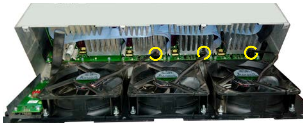
Figure 3: Disconnect the fan wires
