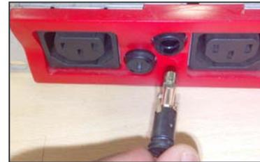
Step 3: Replace the appropriate new Fast Acting Fuse in the holder.
