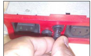
Step 5: By using the Flat Screw Driver gently turn the Fuse holder to 45° in clock wise direction.
