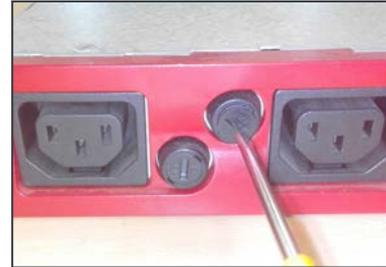
Step 2: Remove the Fuse holder from the slot.
