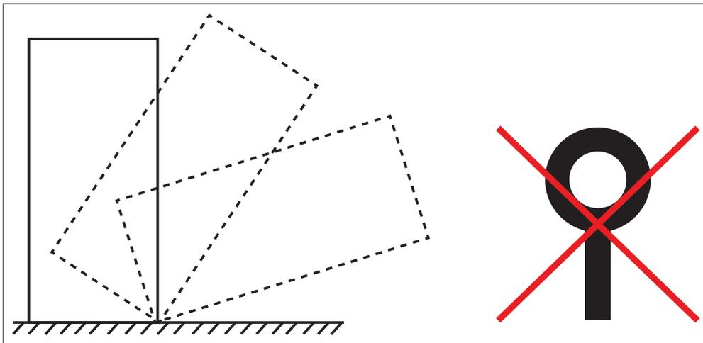
**Warning:** The top cover fixing bolts must NEVER be replaced with lifting eye bolts.
